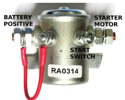
In the early years Ford used two different start buttons and ignition switches, this solenoid can be used for either 1 or 2 wire start buttons by changing the red jumper wire. A one wire start button is ground activated, a two wire is 12 volts activated.
