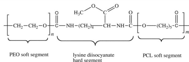
Figure 2: Spandex chemical structure.
