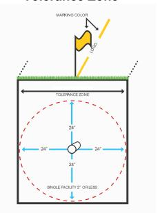
OAR 952-001-0010 (25) "Tolerance Zone" means the area within 24 inches surrounding the outside dimensions of all sides of an underground facility.
