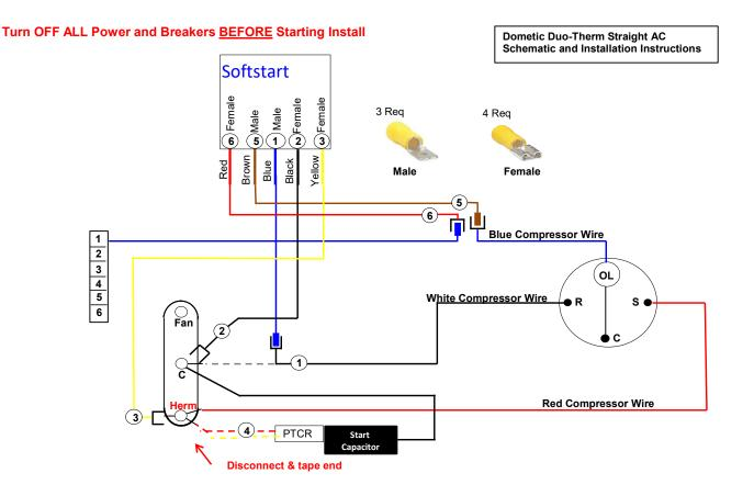
Route Blue, Black and Yellow Softstart wire into electrical Box and crimp disconnect as shown in softstastr drawing above
