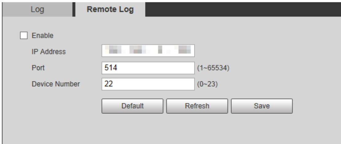
**Step 2** Select **Enable** check box to enable the remote log function.
