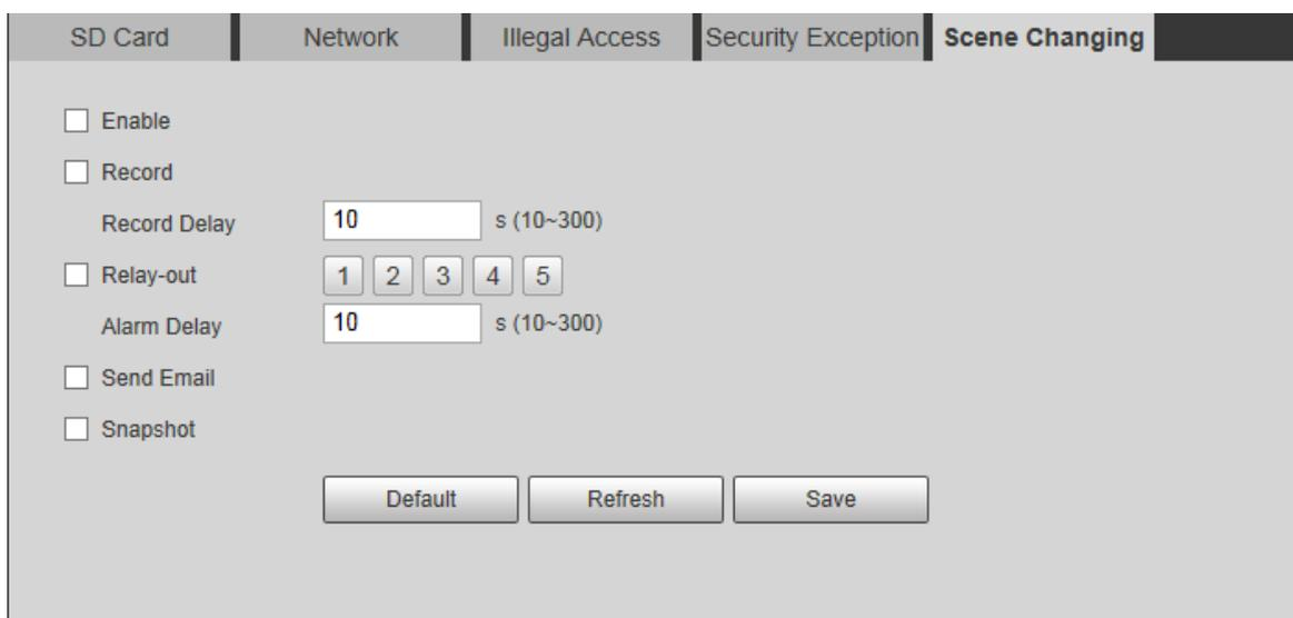
**Step 2** Select **Enable** check box to enable scene changing alarm, and then configure other parameters as needed. For details, see Table 4-18.
