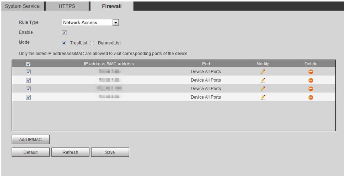
**Step 2** Select **Network Access** from **Rule Type** list, and then select **Enable** check box.
