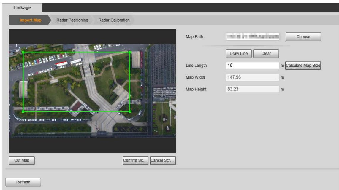
**Step 3** Crop the map according to the detection range of the radar. Drag the box to select the range, and then click **Cut Map**.
