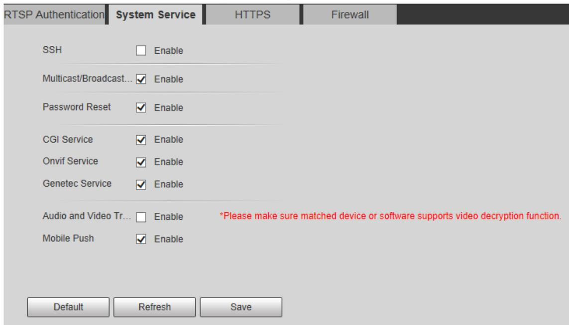
**Step 2** Configure system service parameters. See Table 4-28.
