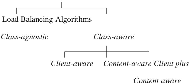
**FIGURE 4.1. General taxonomy of load-balancing algorithms.**
