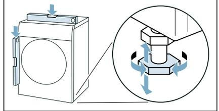
3. Tighten the lock nut against the housing. In doing so, hold the foot tight and do not adjust its height. The lock nuts on all four appliance feet must be screwed tightly against the housing.
