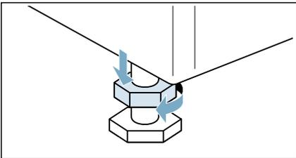
2. Check the alignment of the appliance with a spirit level, and adjust it if necessary. Change the height by turning the appliance feet. All four appliance feet must stand firmly on the ground.
