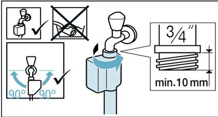
**Tip:** Connect also an external water filter (depending on the model) between water supply hose and tap. The filter filters dirt particles out of the water.
