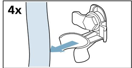
2. Unscrew and remove all four transport brace screws.
