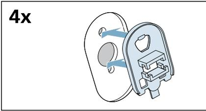
4. Lock the covers firmly in place by applying pressure to the snap-in hooks.
