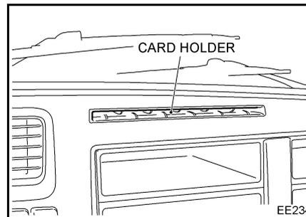
This can be used to hold such cards as telephone cards and highway cards.
