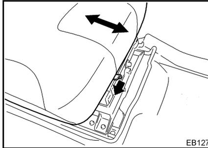
Adjust the cushion to the desired position while pushing the lever to the right. It is possible to adjust in two stages in the forward direction from the standard position.
