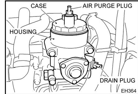
1. Clean outside the filter not to get dust into the filter at the disassembly. Prepare a tray for drained fuel (approx. 2.1 qt [2.0 liter]) and a hose (inner diameter 0.2 in [5 mm], length 3.3 ft [1 m]).
