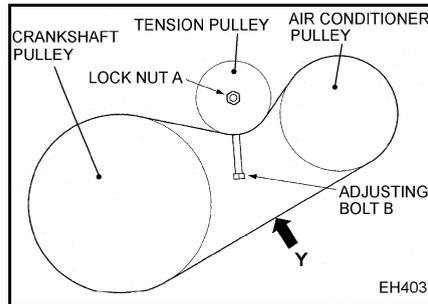
3. After adjustment, securely tighten the lock nut A.
