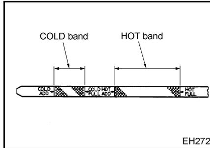
fluid level is within the COLD band range. If the fluid level is not within the range, refill fluid.
