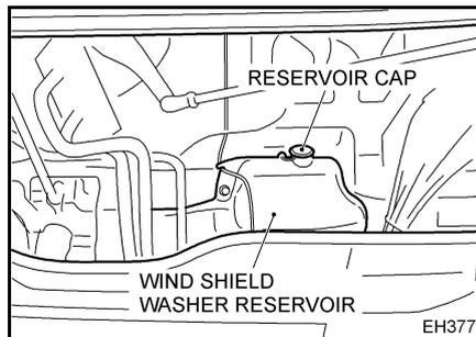
Open the front lid, and check the fluid level in the windshield washer reservoir daily. If low, add an appropriate washer fluid solution. Also, check that fluid is properly sprayed onto the windshield.
