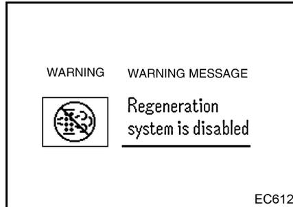
5. When the warning of DPF regeneration by the exhaust gas cleaning device is no longer displayed on the multi-display monitor, manual DPF regeneration is completed. The engine speed at idle will return to normal.
