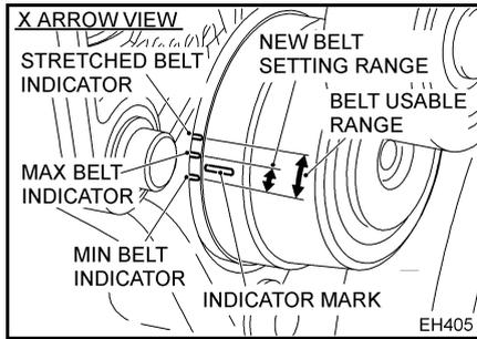
If the indicator (raised line) is out of stretched belt indicator, or if the belt is damaged, replace the belt with a new one.
