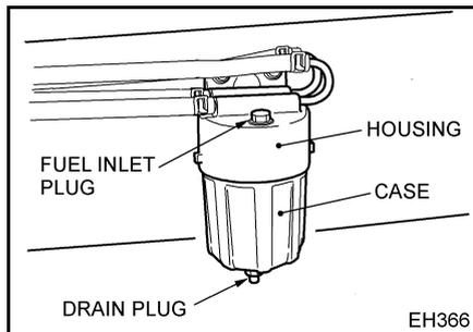
1. Clean outside the filter not to get dust into the filter at the disassembly. Prepare a tray for drained fuel (approx. 2.1 qt [2.0 liter]).
