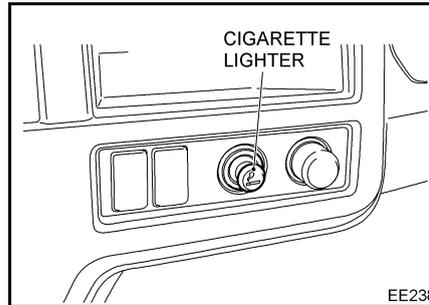
The cigarette lighter is located at the right side of the heater control. To operate the lighter, push it in. The lighter will pop out to its normal position when heated.
