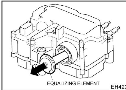
5. Insert the puller, and remove the filter using the puller.
