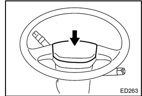
The horn pad is mounted in the center of the steering wheel. Press on the pad to sound the horn.
