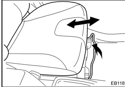
The driver's seat can be adjusted forward and backward by pulling up on the slide lever located on the front of the seat base and sliding the seat to the desired position. Lock the seat in place by releasing the lever. To assure that the seat is properly locked in place, attempt to slide the seat fore and aft with the slide lever released.
