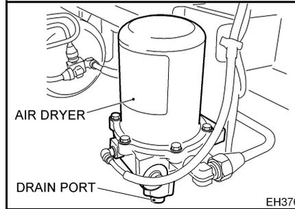
Visually check to be sure that water drains from the drain port of the air dryer. Water will drain when the air pressure governor stops pressurization. The governor stops pressurization when the air pressure in the reservoir reaches the upper level of the normal operating pressure range. When the sound of air supplied to the reservoir can no longer be heard, or when the sound of the engine changes, this condition has been reached.
