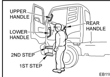
2. Firmly grasp either the lower or upper handle on the front of the door opening with your left hand and place your left foot on the 1st step.
