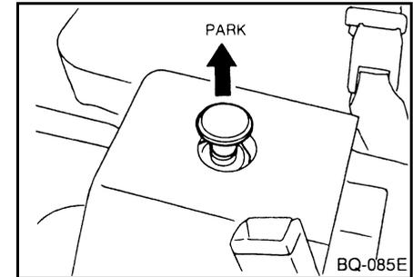
The parking brake valve is located to the rear of the gear shift lever. Pull the knob up to operate the parking brake. When the knob is pulled up, the PARKING BRAKE warning light comes on. To release the parking brake, press the knob down. The warning light will go out.
