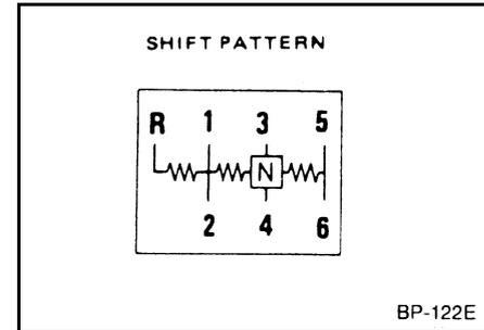
Familiarize yourself and others operating the vehicle with the manual transmission, the gear shift pattern and clutch operation. When using the clutch, be sure that the clutch is fully engaged or disengaged. Never operate the vehicle with the clutch partially engaged.
