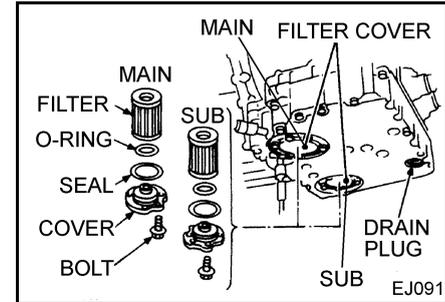
1. Clean the periphery of the filter cover to prevent dust from entering at the time of removal of the filter.
