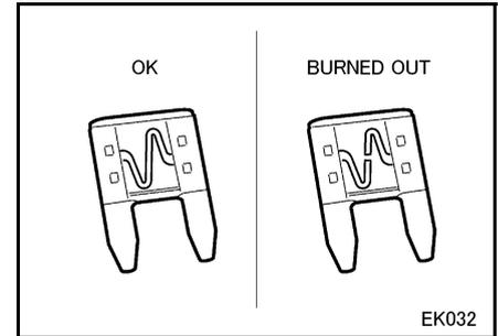
2. Install a new fuse with the same current rating as that specified for the circuit.
