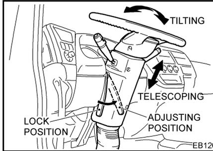
The steering wheel telescopes 2.95 inches (75 mm) and tilt angle 9.5°. Position the driver's seat before adjusting the steering wheel. Loosen the lock lever and adjust the steering wheel to the desired position. After adjustment, securely tighten the lock lever.
