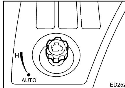
The engine throttle control knob, located to the left of the steering column, can be used to adjust engine idling speed. Normal engine idling speed is 550 rpm. If equipped with automatic transmission, make sure the engine idling speed is 550 rpm at the forward range.
