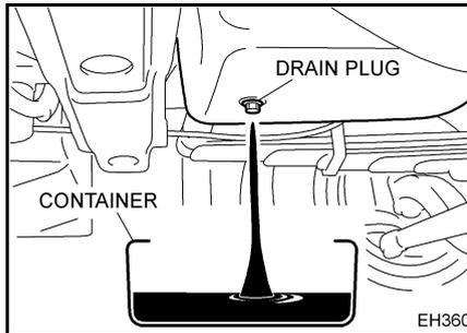
4. When all the oil has been drained from the oil pan, replace the drain
