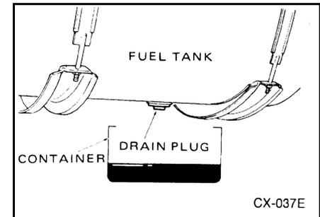
3. Allow all the water to drain from the tank.
