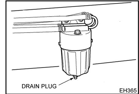
1. Stop the engine, prepare a tray to receive drained water.
