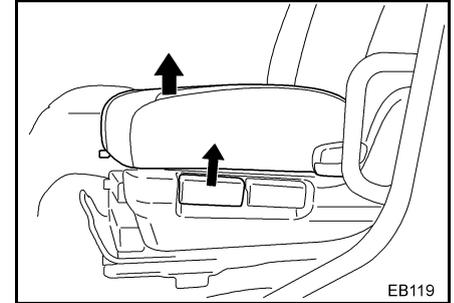
The front of the driver's seat can be raised by pulling up the lever at the left side of the seat base. To lower the seat downward, pull the lever and push down on the seat.
