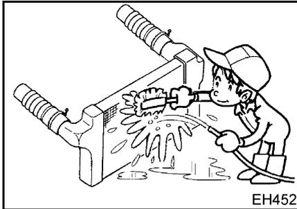
The charge air cooler is used to cool the overheated intake air charged by the turbocharger, and is installed at the front of the radiator.
