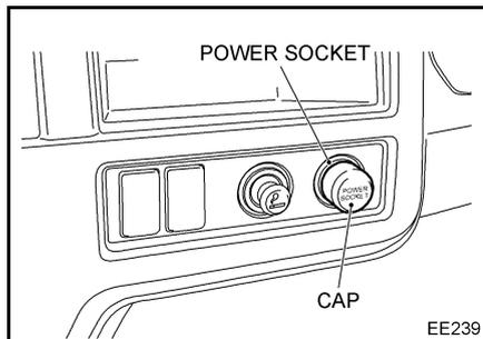
The power socket is located at the right side of the cigarette lighter. Use the power socket in the cab to connect commercially available car accessories. Remove the cap before use. The following devices can be connected to the socket.
