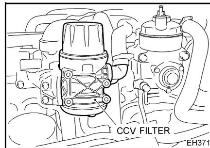
1. Clean the area around the CCV filter cap to prevent dirt from entering during replacement.
