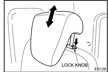
The height of the headrest can be adjusted manually. Adjust the headrest height while pressing the lock knob.
