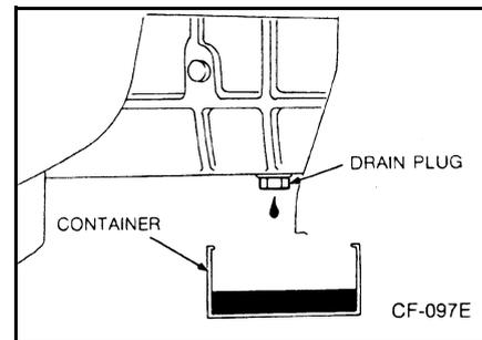
2. After draining, replace the gasket of the drain plug with a new one. Reinsert the plug and tighten the plug.
