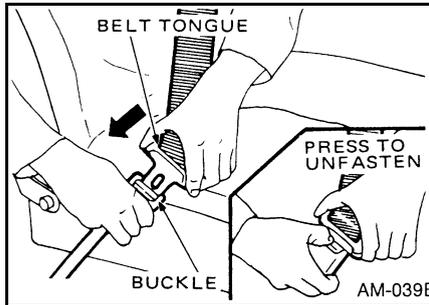
To fasten the belt, position the seat and fit the seat belt snugly without twisting. Insert the open end of the tongue into the buckle until it snaps and engages.
