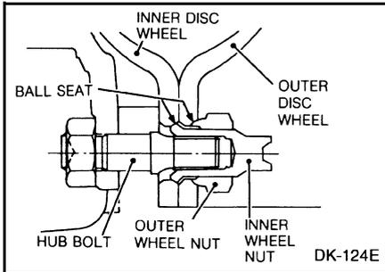
1. Loosen the outer wheel nuts.
