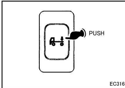
This switch is located at the right side of the heater control. By operating this switch, the vehicle bed can be lowered by exhausting air from the air spring at the rear axle to facilitate loading/unloading work.
