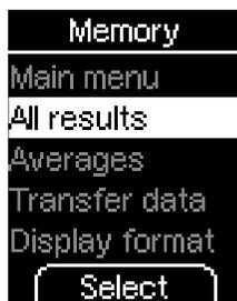
In addition to the result, the time and the date, your meter also saves all other information that is relevant to the test. This includes all symbols displayed with the result after a test (except the battery symbol) and the flags you added to the results.
