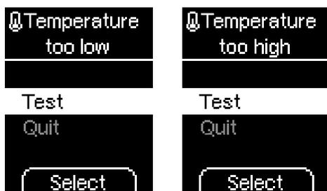
**Temperature too low / too high:** This message appears at the start of a test if the ambient temperature or the temperature of the meter is between +8 and +10 °C or between +40 and +42 °C.
