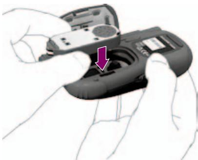
**7** Insert the cassette in the meter with the silver side facing upwards.
