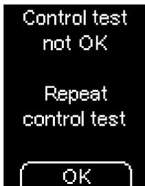
If *Control test not OK ... Repeat control test* is displayed, the result obtained is not within the concentration range displayed. Check the points listed on the next page. If your answer is different from the answer given, make the respective corrections and repeat the test. If you have taken all of these points into account and *Control test not OK* is still displayed, contact Accu-Chek Customer Care.
