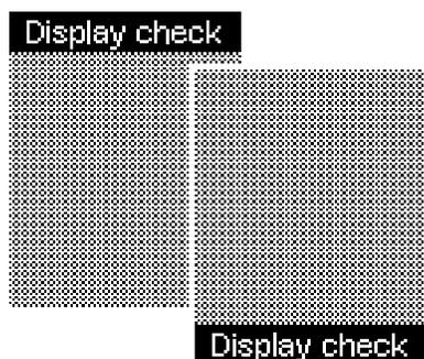
The meter then runs a display check in which a black and yellow checkerboard pattern of small illuminated dots is displayed.
