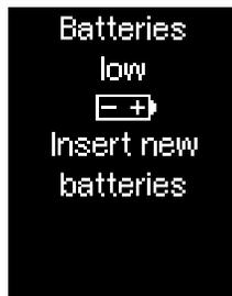
**Batteries low:** This message appears when the batteries are almost empty. It appears every time you turn the meter off until you change the batteries. The first time the message appears, you can still perform about 50 tests.
