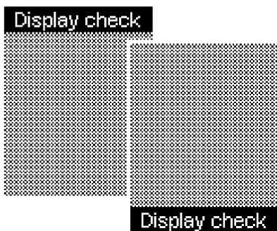
The meter first runs a display check in which a black and yellow checkerboard pattern of small illuminated dots is displayed.
