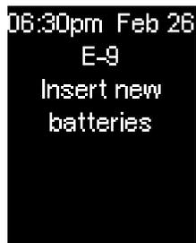
If the batteries are so low that no more tests can be performed, this message will appear. Then the meter turns off (after a maximum of 1 minute).
