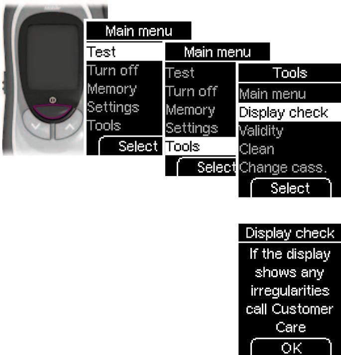
If you wish to check whether the display is working properly, in addition to turning on the meter, you can also do this via the display check in the *Tools* menu. In this case, the display check is shown until you cancel it (for no longer than 1 minute).
