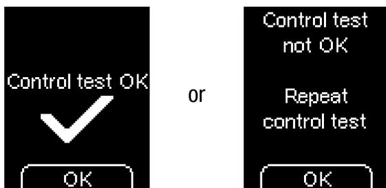
If the result is within the concentration range displayed, *Control test OK* is displayed.
