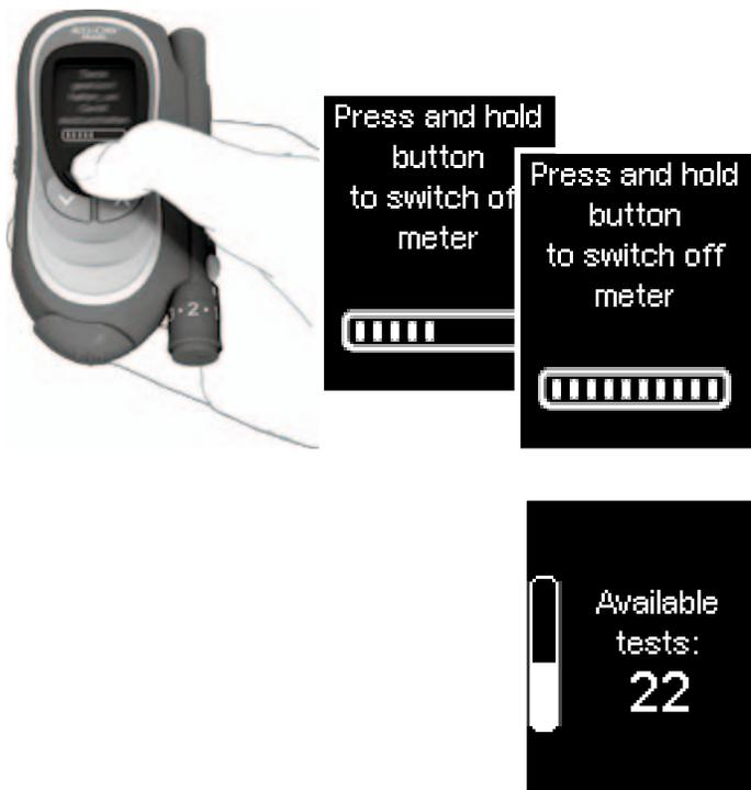
There are 2 different ways of turning off the meter: using the On/Off button
