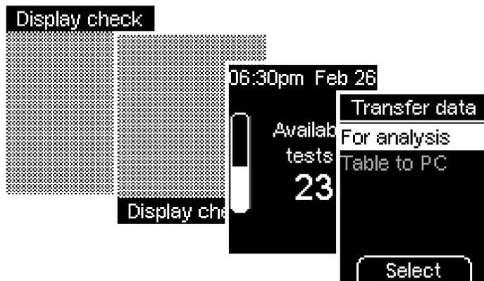
After the display check and the number of available tests, the *Transfer data* menu is displayed.
