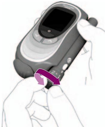
You can set the penetration depth of the lancet to 1 of 11 possible settings (0.5–5.5). The silver line (depth setting indicator) on the lancing device indicates the current penetration depth setting. The higher the number the deeper the penetration. The half settings for the penetration depth are indicated by a dot. The penetration depth 1.5 is set when the line points to the dot between 1 and 2.
