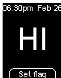
If the result is higher than 33.3 mmol/l, **HI** is displayed instead of a result. Repeat the test.
