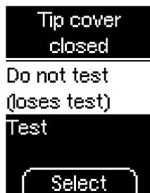
**Tip cover closed:** This message appears if you close the tip cover after the meter has advanced a test area.
