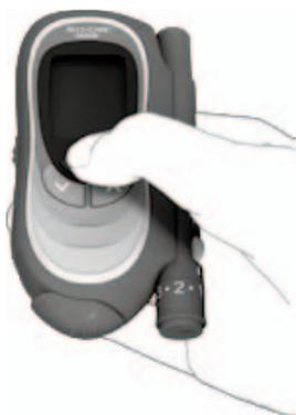
With the meter off, press and hold the On/Off button
