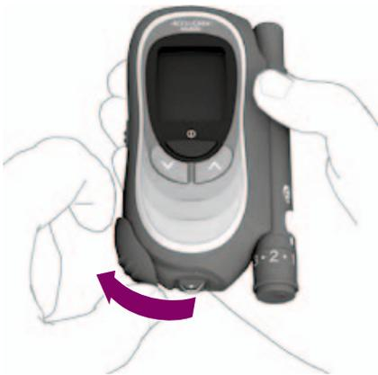
Start as for a blood glucose test: Either open the tip cover or select *Test* in the *Main menu*.
