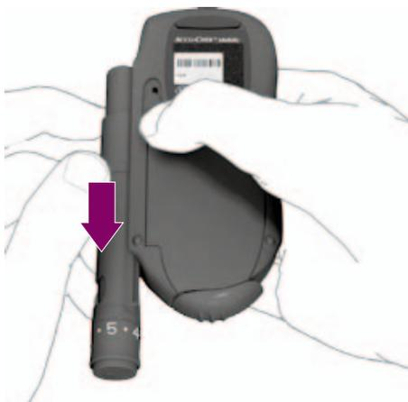
**2** Withdraw the lancing device by sliding it out in the direction of the arrow.
