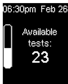
You can view the number of tests still available on the inserted cassette by one press of a button.
