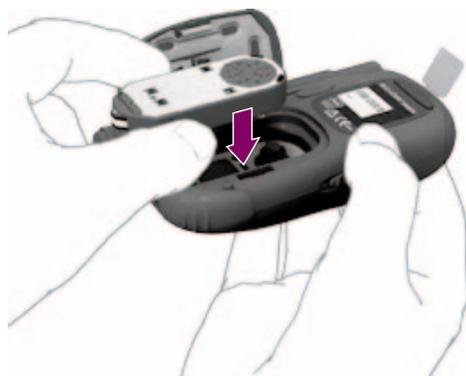
**6** Insert the cassette in the meter with the silver side facing upwards.
