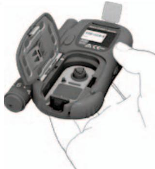
The cassette compartment cover is fully opened when it is at an angle of slightly more than ninety degrees – as shown in the illustration.
