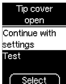
**Tip cover open:** This message appears if you are in the process of changing a setting (e.g. the date) or entering a new setting (e.g. a reminder) and open the tip cover.
