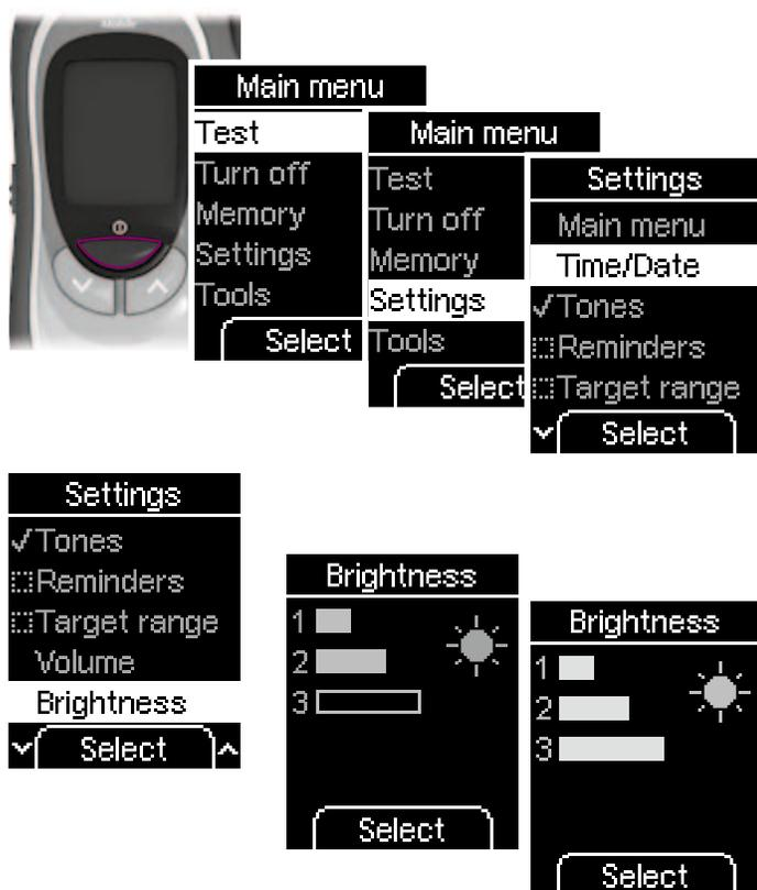
You can set the brightness of the texts and symbols appearing on the display to one of 3 different levels.
