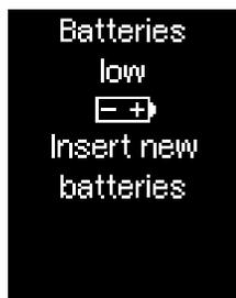
This message appears when the batteries are almost empty. It appears every time you turn the meter off until you change the batteries. The first time the message appears, you can still perform about 50 tests.
