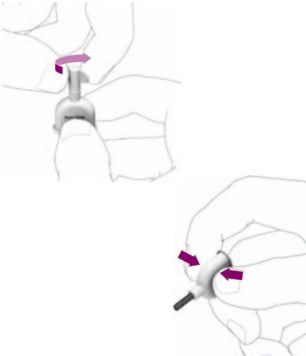
**3** Twist the cap off the applicator. Be careful not to squeeze the applicator too hard while doing this so as to not lose any control solution.
