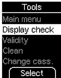
The *Tools* menu on the one hand offers you some extra means of checking the meter. On the other hand, you must also use this menu to prepare for cleaning the meter and changing a test cassette that has not been used up.
