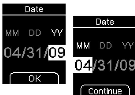
**i** If the date you have set does not exist (e.g. April 31), the meter returns to the first setting position when you confirm the last entry with *OK* (step 7). You must correct the date before the meter will accept it.
