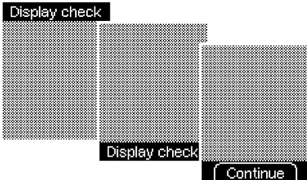
When you have closed the cassette compartment cover, the meter turns on again and runs the display check.
