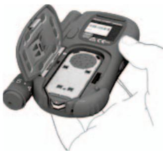
The cassette compartment cover is fully opened when it is at an angle of slightly more than ninety degrees – as shown in the illustration.
